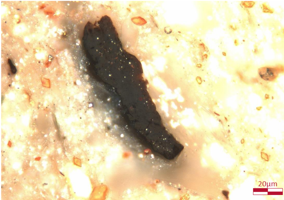
Sample 6126527243 (4485') : Representative vitrinite particle with a reflectance reading of 0.49%Ro from central measuring circle.
