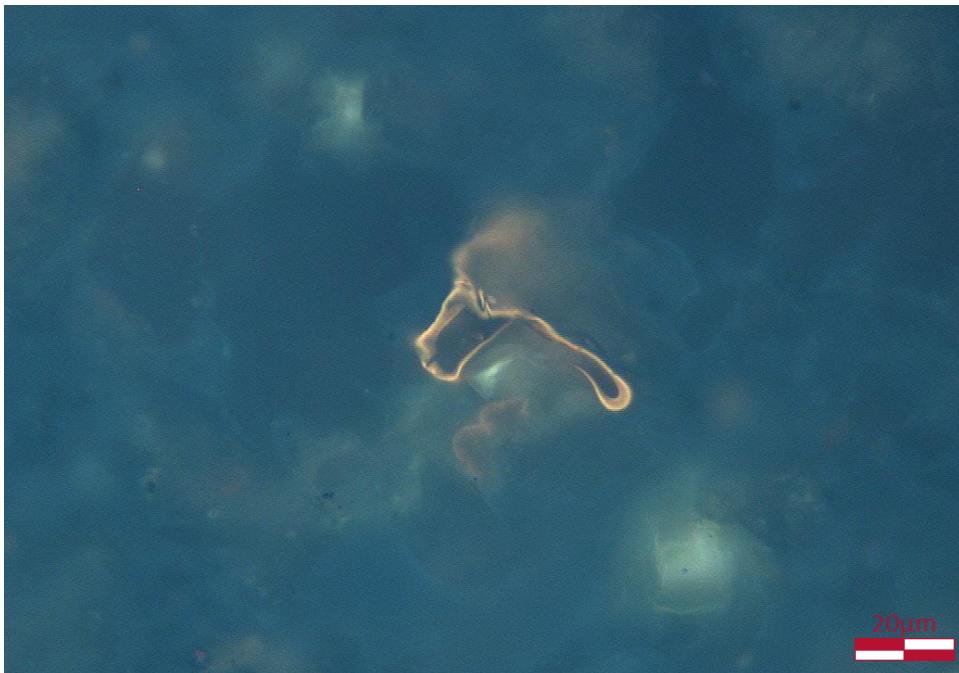
Sample 6126527261 (8917): Orange fluorescing spore(?) (reworked) within the same sample suggesting a maturity estimate of 0.7-0.9%VR/e.
