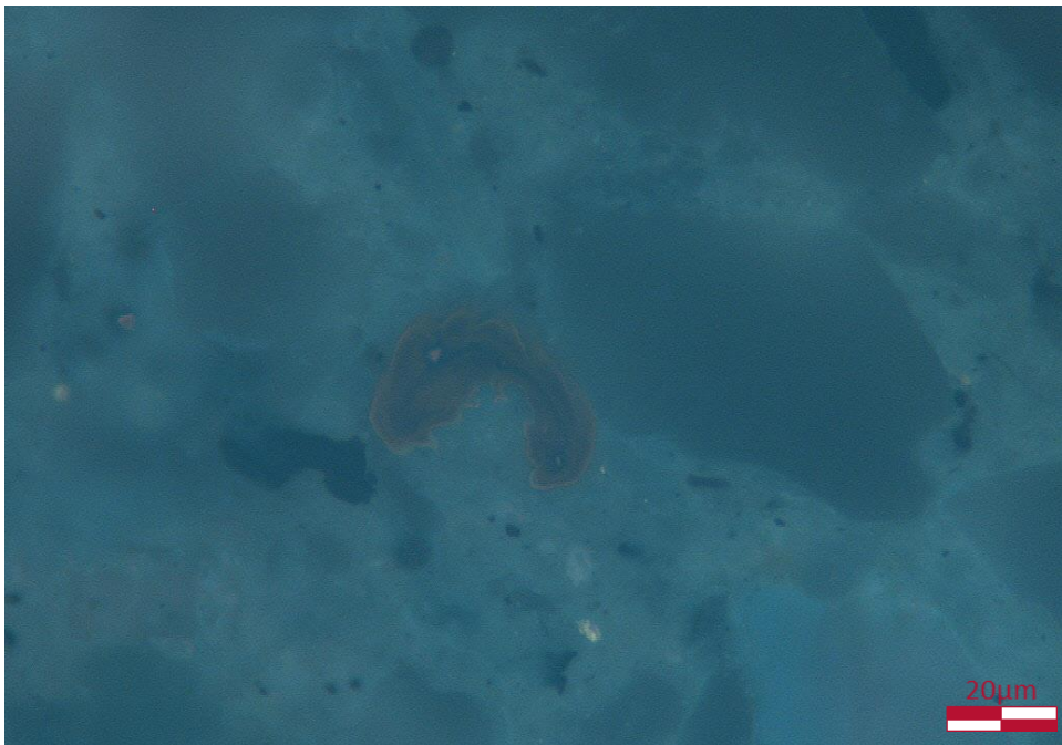
Sample 6126527251 (7503') : Identical field of view as previous photomicrograph under UV light revealing dull orange to light brown fluorescence from spore suggesting a maturity estimate of 0.8-1.1% VR/e.
