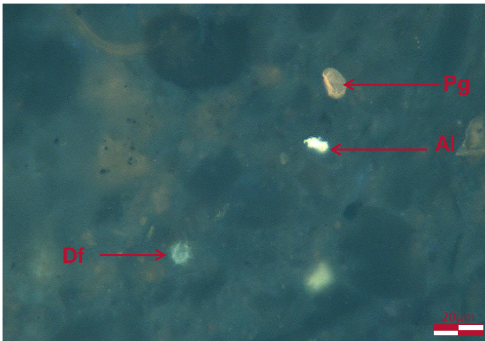
Sample 6126520998 (9180') : Variation in liptinite fluorescence colours from weak greenish yellow dinoflagellate (Df), yellow algal debris (Al) and orange pollen grain (Pg).
