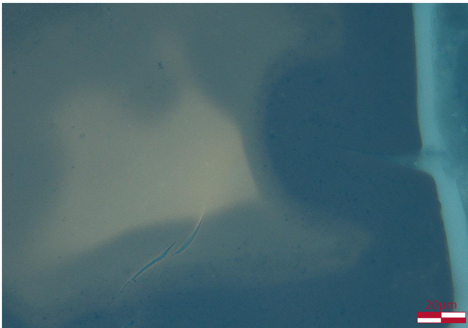
Sample 6126527253 (7705') : Dull orange fluorescence from centre of bitumen particle with distinct reductions in intensity moving towards perimeter (effects of biodegradation???)
