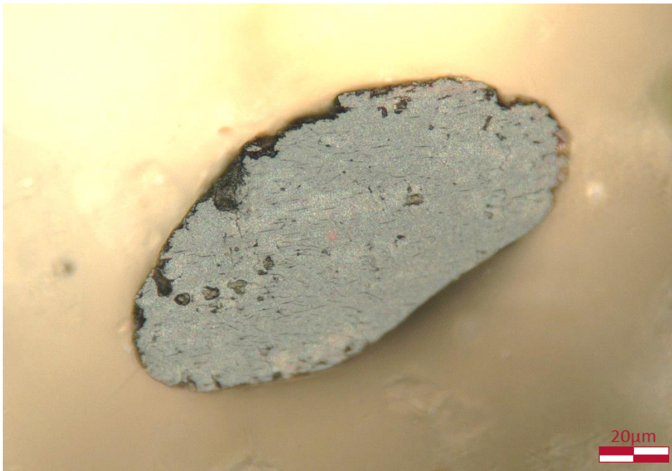
Sample 6126520962 (1740') : Oxidised vitrinite particle. No representative vitrinite is present in this sample.
