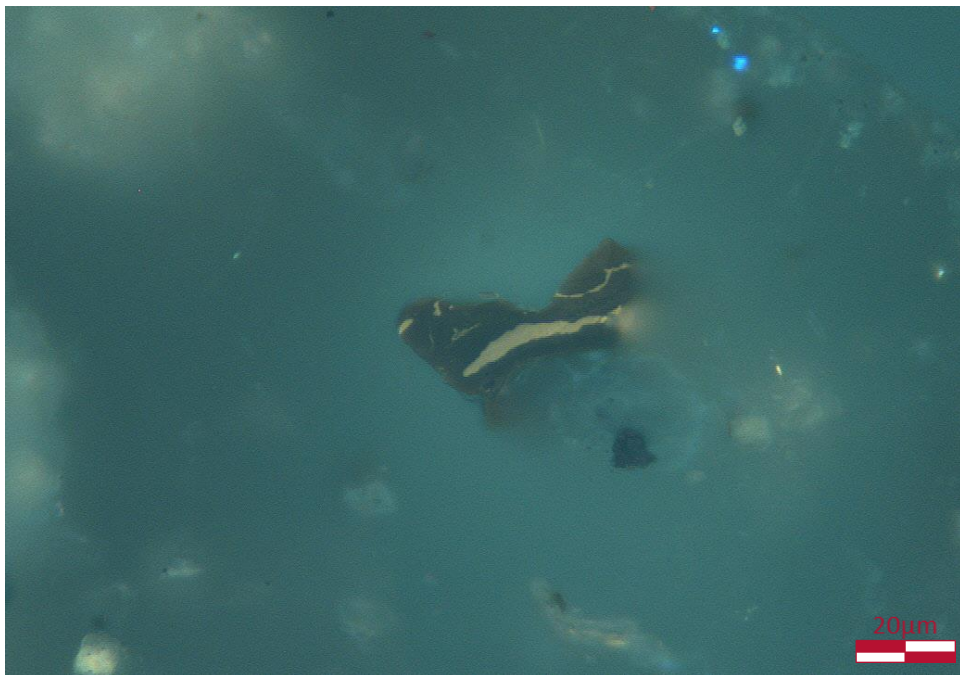
Sample 6126520988 (8280') : Note weak brown fluorescence from vitrinite associated with reflectance suppression.
