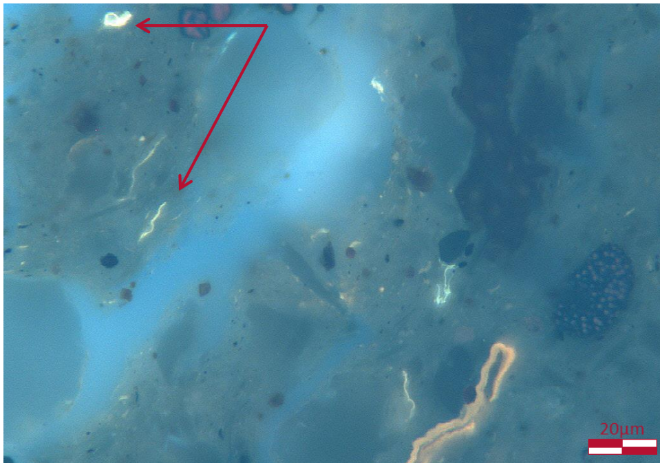
Sample 6126527243 (4485') : Scattered yellow fluorescing microplankton (indicated). Rare orange fluorescing cutinite, considered reworked, is also present (bottom right).
