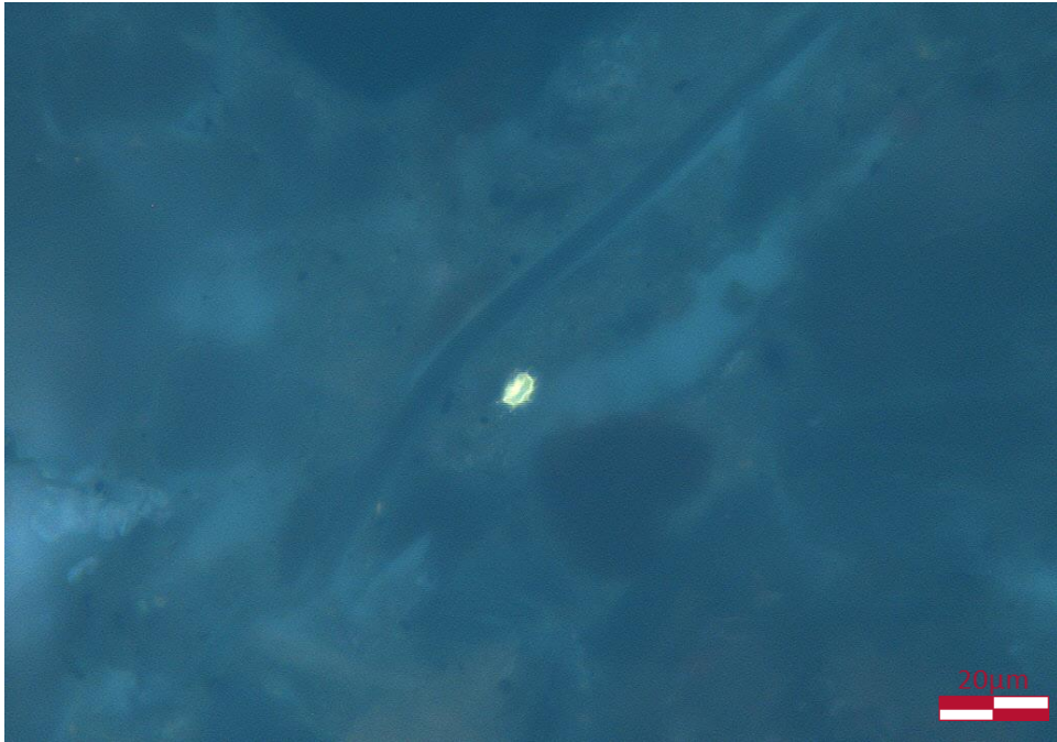
Sample 6126527245 (6132') : Isolated yellow dinoflagellate (interpreted autochthonous). Yellow colour suggests a maturity estimate of 0.4-0.6% VR/e.
