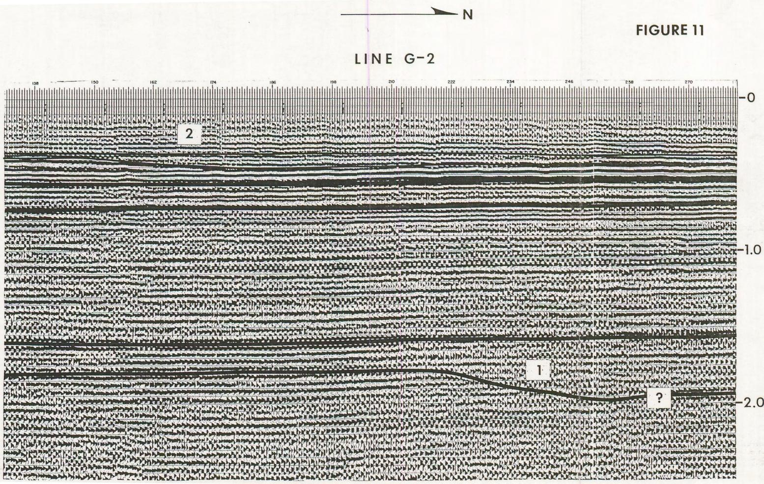
Gravity and magnetic data also possibly support an intrusive body at this location and at locations to the north within the area of study (Watkins, et al., 1985). Here erosional relief is positive.
