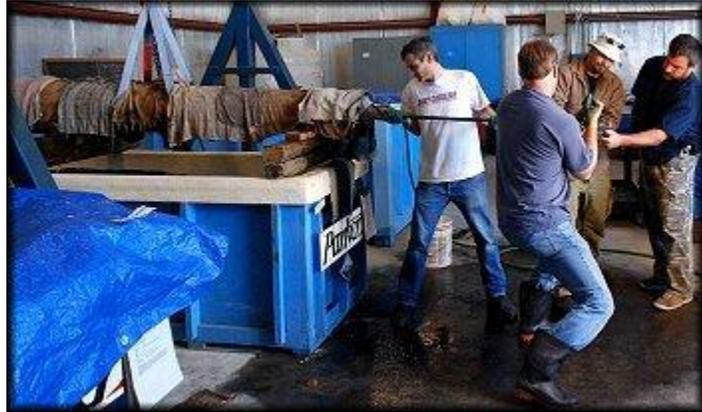
To facilitate drilling out the remaining concretion within the bore of Cannon **2**, we obtained the diameter at the muzzle opening and 9 inches into the bore measuring four different directions, vertically, horizontally and diagonally. The bore's diameter seemed to be 3.8"-4.0", so we
