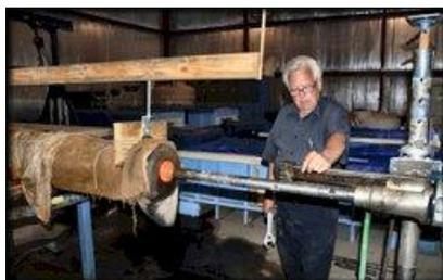
A horizontal core drill was rented from Kore Kut and Mr. John McClain showed us how to use the equipment. As the core drill advances water is pumped into the core to reduce friction and some of what is removed is flushed out to give you an idea of what you are drilling into. The core drill was set up level with the bore of the gun and we started slowly advancing the bit
