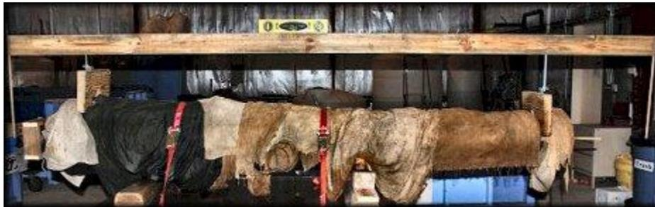
ordered a 3.75" core bit. Before any drilling took place we had to make sure the bore was level. We built a leveling apparatus that sat on top of the gun. A round wooden cut out with a dowel rod in the center was
