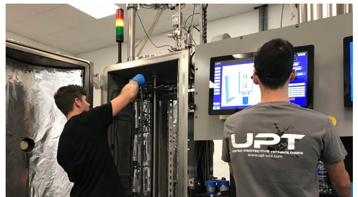
Sam Efrid, Chemist, and Alan Pope, Lead Production Technician, loading components to be coated, and verifying the correct deposition recipe.
