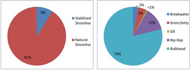
Figure 87: Percent stabilization structure by structure type.
