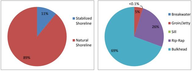
Figure 23: Percent stabilization structure by structure type.
