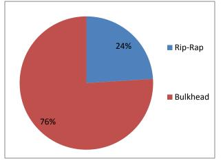
Figure 18: Shoreline stabilization structures that are coincident with the shoreline for North Carolina.
