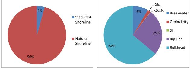
Figure 39: Percent stabilization structure by structure type.
