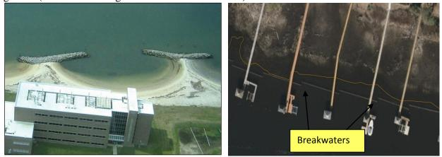
Figure 7: Examples of breakwaters from aerial photographs.
