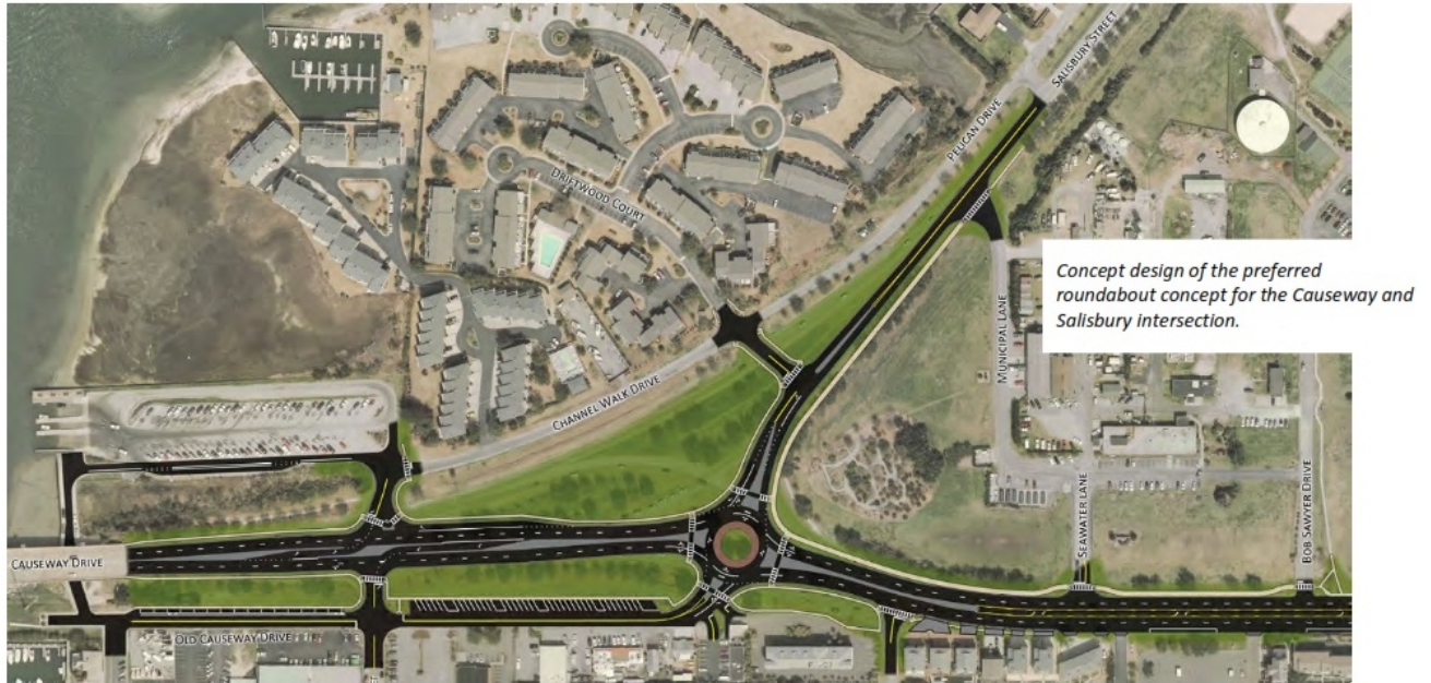
Conceptual Design for Causeway Drive/Salisbury Street Image Source: Wrightsville Beach Community Transportation Plan
