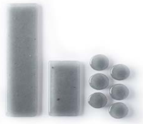
Glass tiles for residential use made from CRT glass
