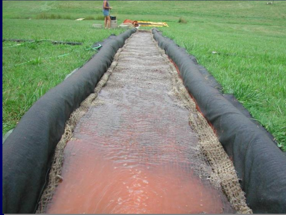
PAM sprinkled on erosion control matting down a slope
