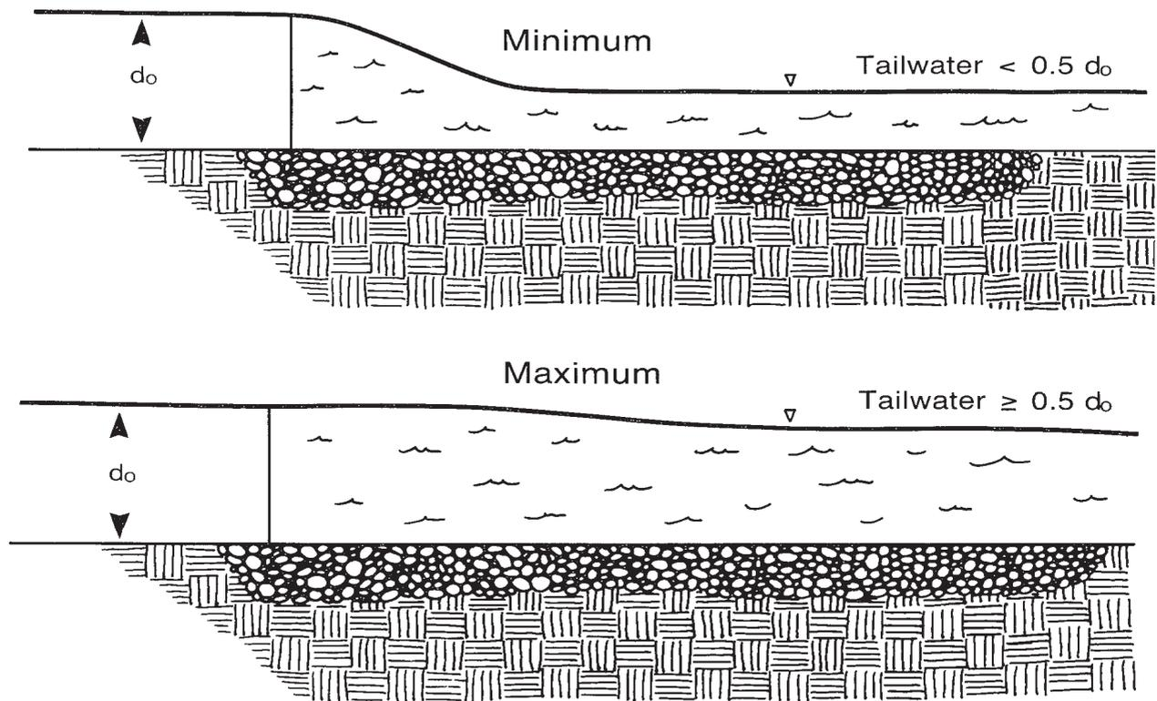
Figure 6.41b Stage showing maximum and minimum tailwater condition.
