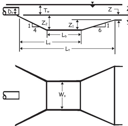
**Riprap Aprons size**—The apron length and width can be determined according to the tail-water condition. If the water conveyance structure discharges directly into a well-defined channel, extend the apron across the channel bottom and up the channel banks to an elevation of 0.5 foot above the maximum tail-water depth or to the top of the bank, whichever is less (Figure 6.41c).
