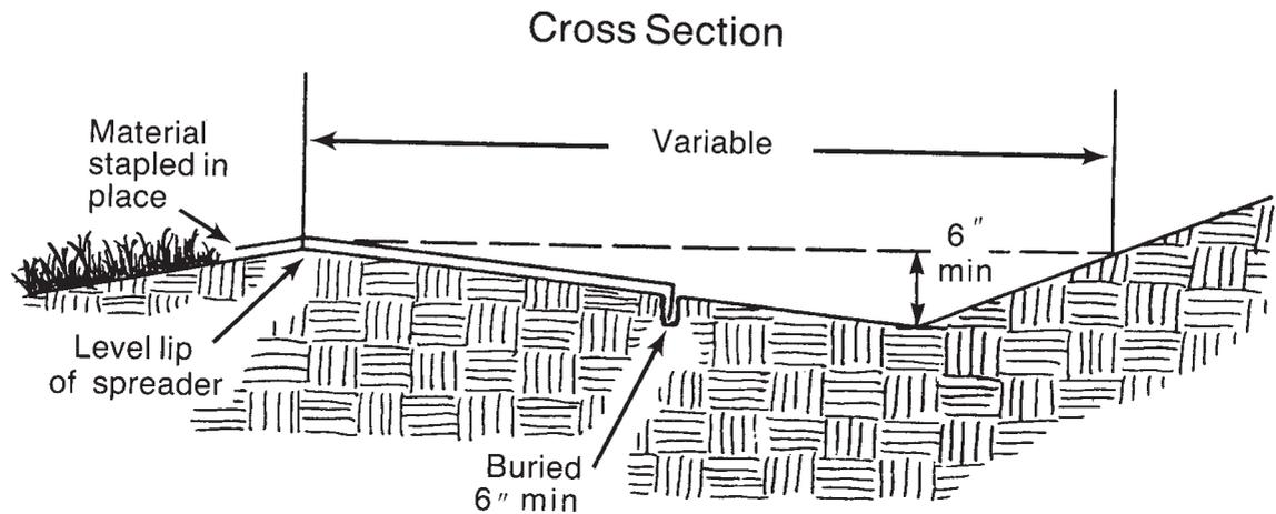
Figure 6.40b Detail of level spreader cross section.
