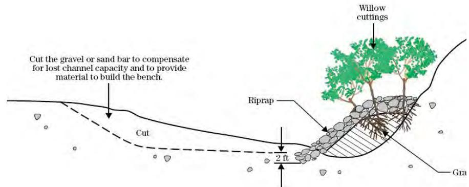
Figure 6.73b Embankment bench method
