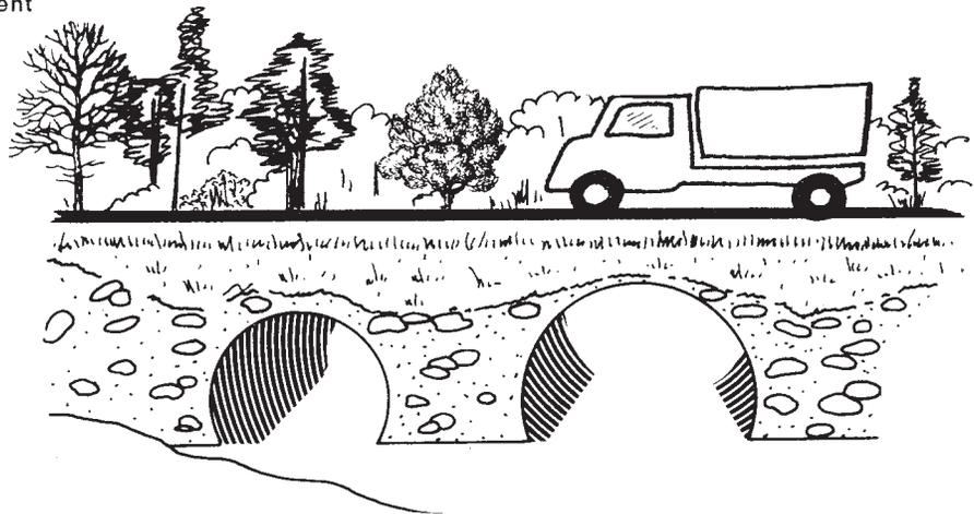
**Design Criteria** Design permanent stream crossings in accordance with N.C. Department of Transportation standards and specifications, considering maximum loadings anticipated, safety, flow capacities, and other requirements for DOT installation approval. The local DOT can provide necessary guidance.
