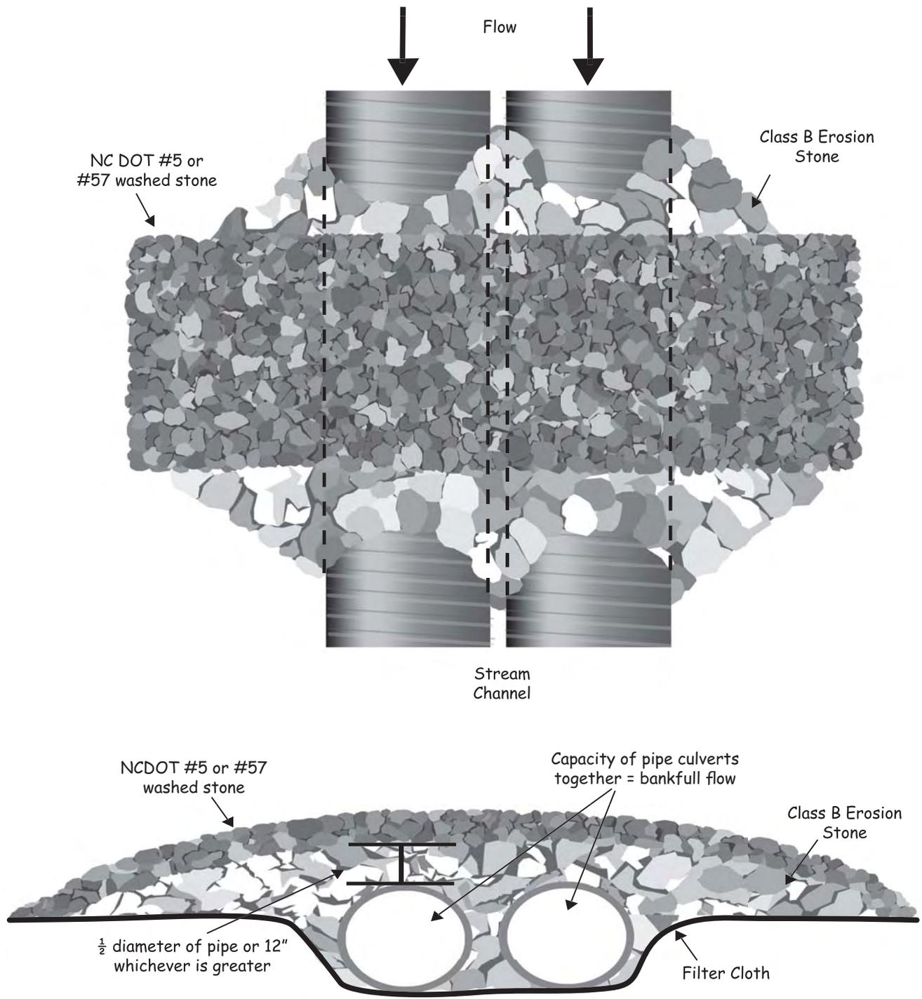
Figure 6.70b Temporary culvert backfilled with stone.
