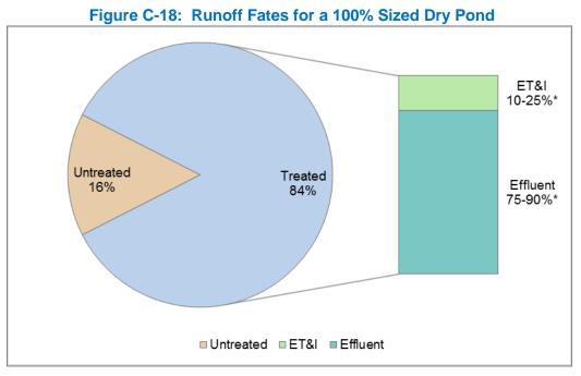
\* NOTE: The percentages of ET&I and Effluent vary based on HSG.
