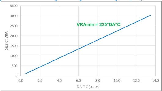
Figure C-15: Minimum Sizing for the Vegetated Receiving Area (VRA) of an LS-FS
