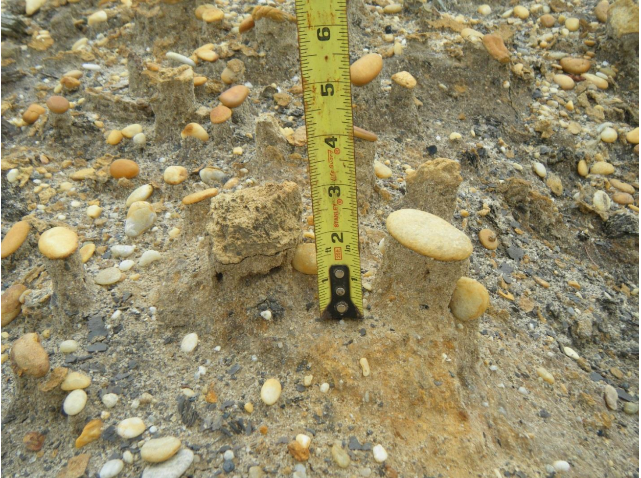
Figure 12. Pebbles have protected the underlying pillars of soil from eroding at site WRO-063.
