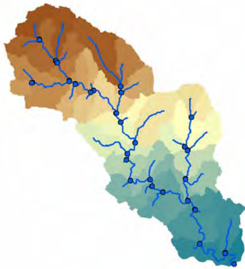
Figure 2.8.3 - Drainage areas, stream segmentation, drain points
