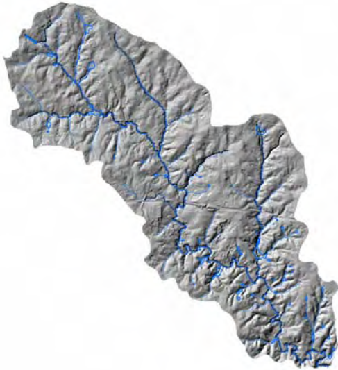
Figure 2.8.1 - Reconditioned DEM, using “Agree” function
