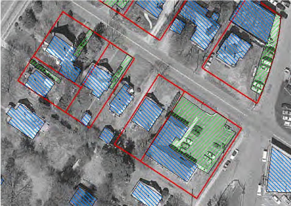
Figure B-2. Example of Sampled Parcels, Building Planimetrics, and Digitized Extra Impervious Areas
