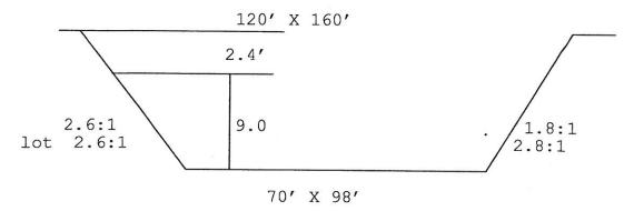
Waste Storage Pond #3 (Parlor Wash Water Pond)"AS BUILT" - The maximum pump out marker is 1.6' below top of dam.
